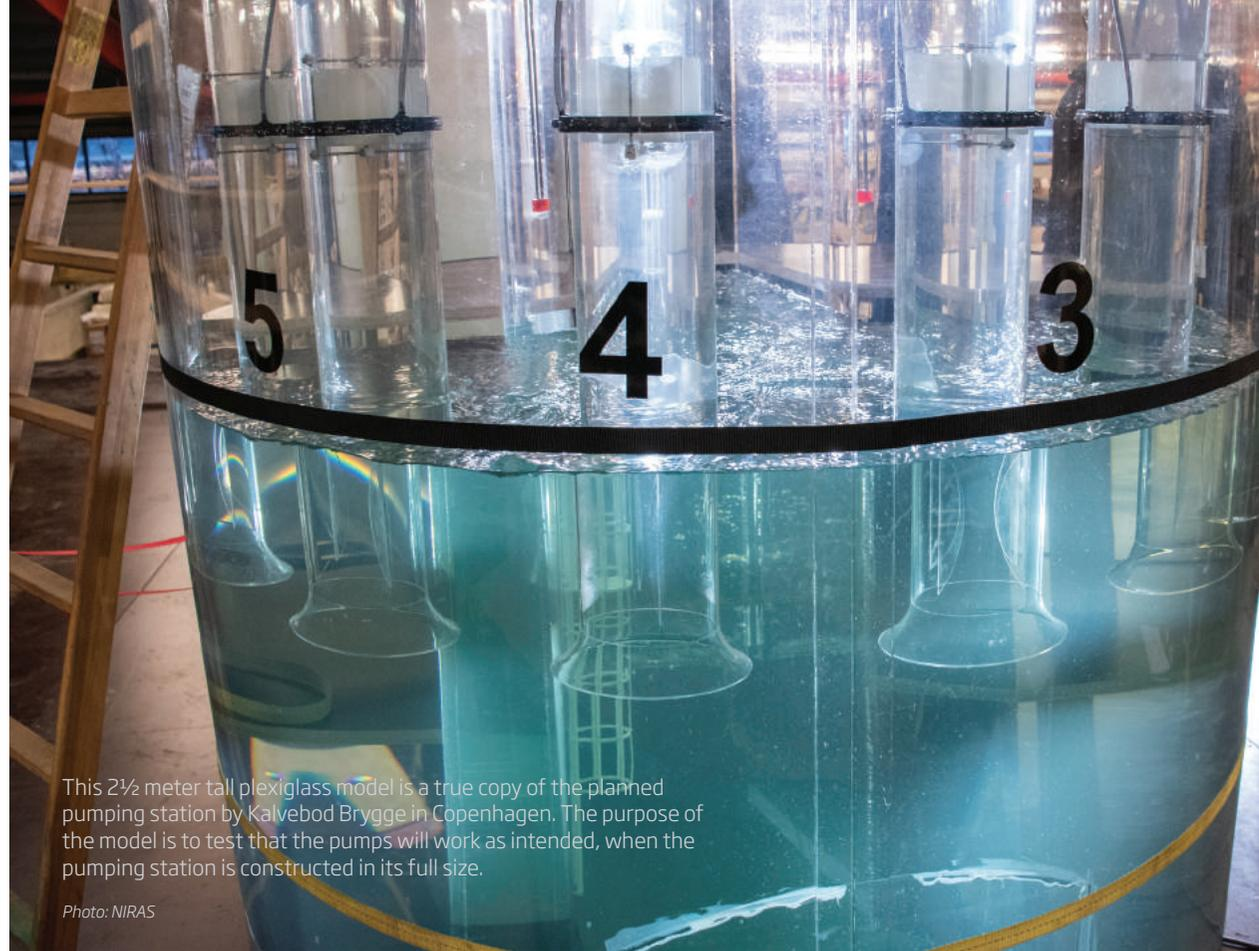
This 2½ meter tall plexiglass model is a true copy of the planned pumping station by Kalvebod Brygge in Copenhagen. The purpose of the model is to test that the pumps will work as intended, when the pumping station is constructed in its full size.
