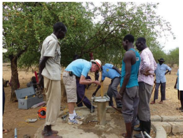
*W4EE team member Mike Wood provides hand-pump management training in Napotpot, Kapoeta East County, Kapoeta State, to measure static water level in boreholes as part of groundwater monitoring.*
