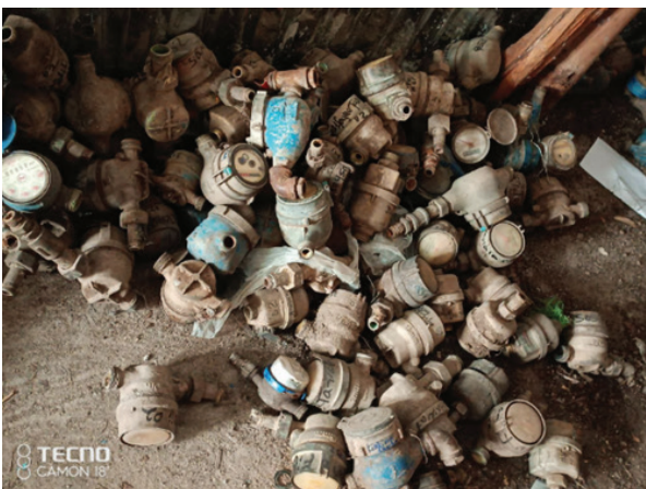
Figure 1: Old and non-functioning water meters collected from customers
