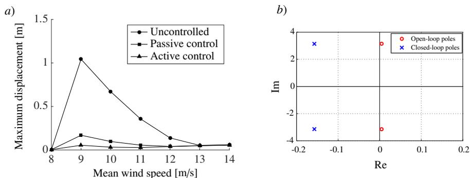
Fig. 3: Performance of the active modal controller. a) Peak cable response under different mean wind speeds with and without control. b) Open-loop poles and closed-loop poles of the 1st cable mode,  $U_0=9$  m/s.
